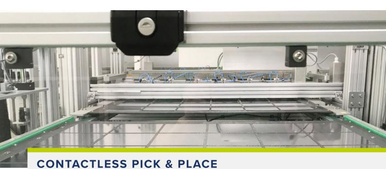
With the Levi-Loader, several solar wafers can be picked up and transported simultaneously without any contact. Precise positioning of wafers on the matrix tray by linear motors or belts with pins is possible as well.
